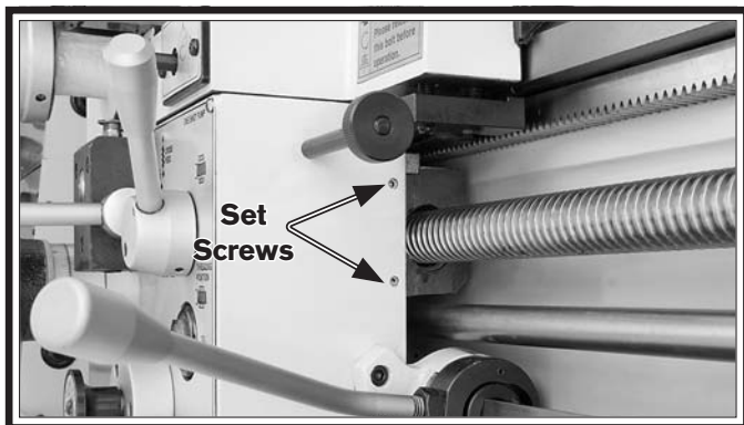
Figure 122. Half nut gib adjustment.
